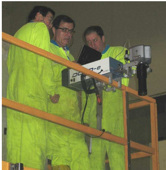
Figure 1. DCVD mounted on fuelling machine at Ringhals nuclear power plant fuel bay
