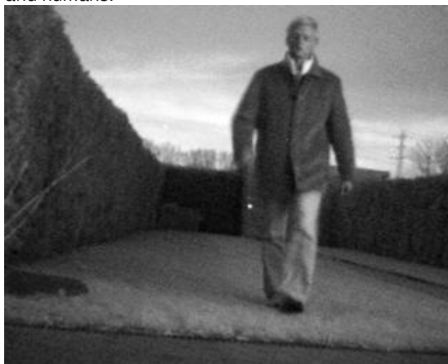
Fig. 1: Nightvision with SWIR InGaAs camera XEVA 1.7 320 TE1 -picture taken at midnight, partly cloudy, few stars, no illumination used-
